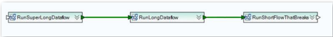
Figure 19. Job Restart allows a workflow to be started from a specific point.
